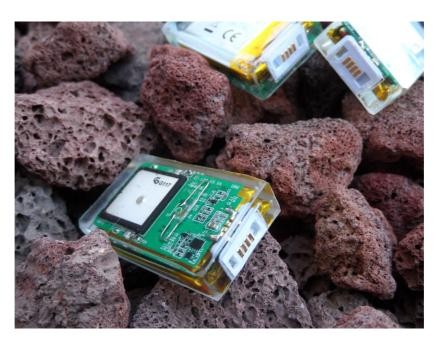
Other than devices in ThermoSeal, which are hermetically sealed, Epoxy potted devices have their interface exposed to the environment. This requires a different type of connector.
