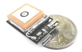
Used in thousands of GPS tags around the world CatLog became the standard GPS data recorder for wildlife bio-tagging.
