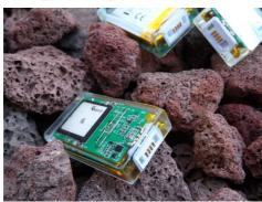
**Epoxy potting** is used for devices that are required to withstand high water pressure and/or mechanical stress like puncturing.
