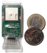
The **ThermoSeal** enclosure offers the best environmental protection for the least weight. It is a special heat shrink tubing with outstanding characteristics.
